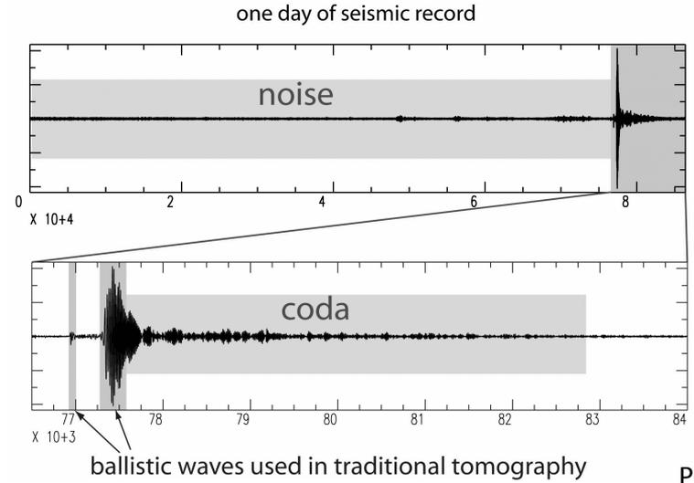
Exploiting the statistical coherence in space and time of continuous waveforms records from dense arrays of broadband and strong motion instruments
