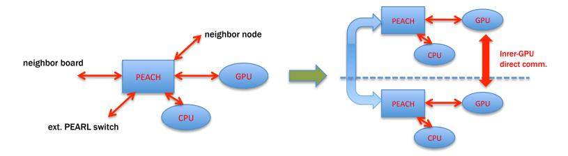
Conceptual image of GPU-direct communication by PEACH (PCI-E Adaptive Communication Hub) utilizing PCI-E link for GPU-GPU, GPU-CPU and node-node communication
