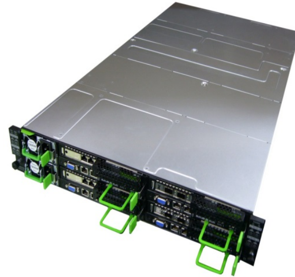
Chassis with 8 nodes, 2U size
