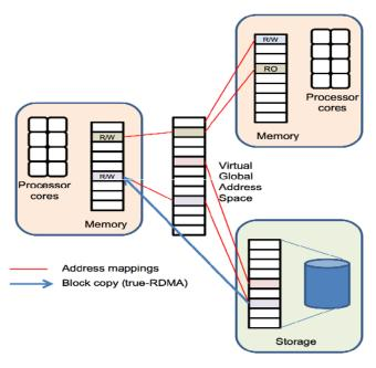
Figure 3 Mapping to global address space
