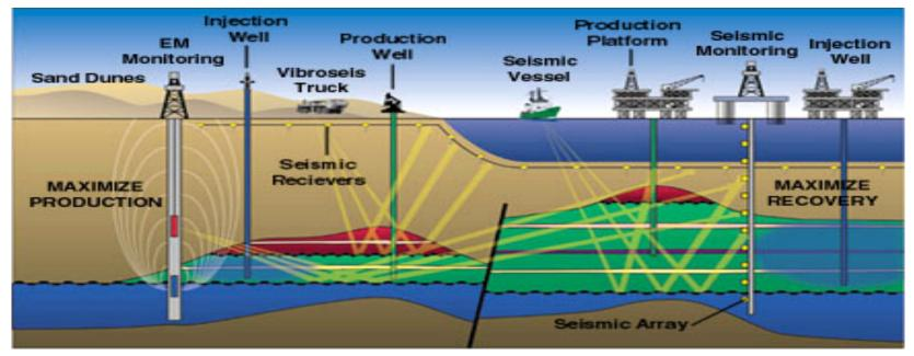
Detect and track changes in data during production Invert data for reservoir properties Detect and track reservoir changes
