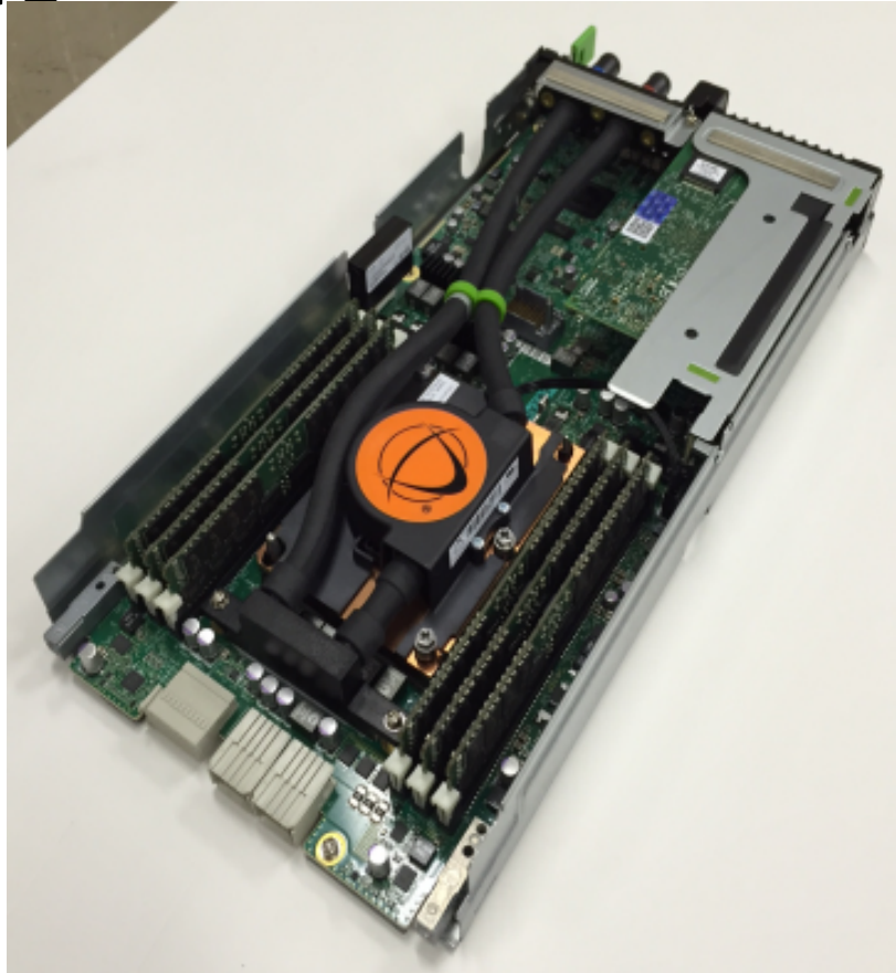
Computation node (Fujitsu next generation PRIMERGY) with single chip Intel Xeon Phi (Knights Landing, 3+TFLOPS) and Intel Omni-Path Architecture card (100Gbps)
